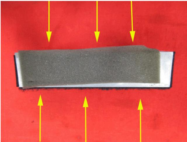
5. Cover the back of the module with 3M™ 4314 Urethane Foam ( $\frac{1}{2}$ " x 7") or equivalent as shown above.
