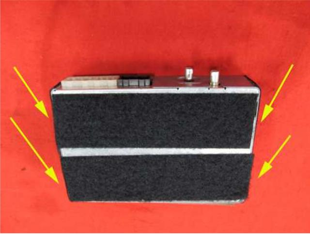
2. Obtain two strips, approximately 177 mm (7 inches) in length, of 2" Velcro® 191195 Reclosable Loop Fastener Tape (hook and loop) or equivalent and apply one side of the tape to the bottom of the module as shown above.
