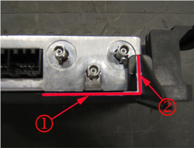
Remove only enough material from the lower edge (1) and shoulder (2) from the bracket to allow the module to seat fully.
