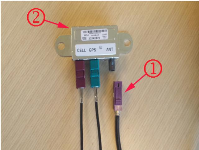
6. Connect the antenna cable (1) from the vehicle to the “upgrade” splitter (2).
