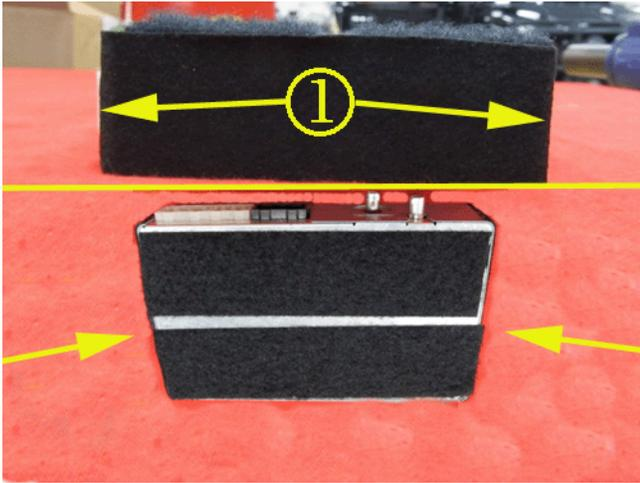
4. Cover both sides of the module with BRS Tape KT13487 (1) or equivalent, as shown above.
