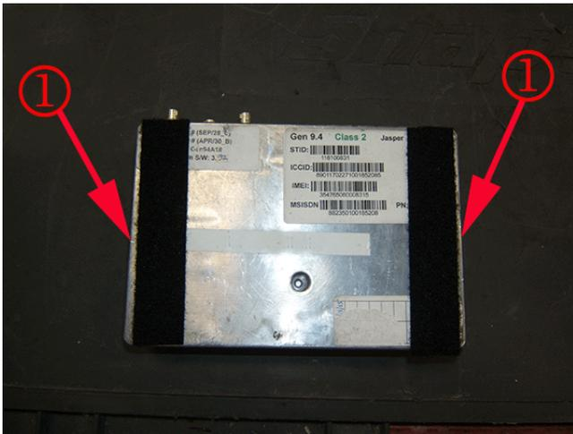
Install one side of 2" Velcro® 191195 Reclosable Loop Fastener Tape (hook and loop) or equivalent as shown above to the new OnStar® module.
