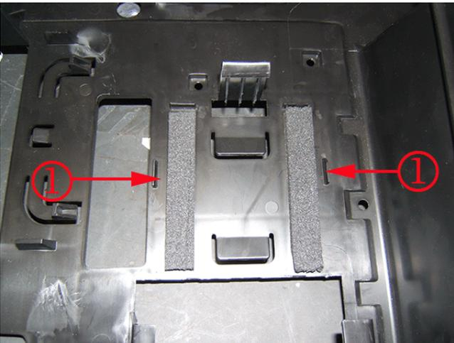
Install the OnStar® module and secure the module with nylon wire tie as illustrated. Trim the excess wire tie material.
