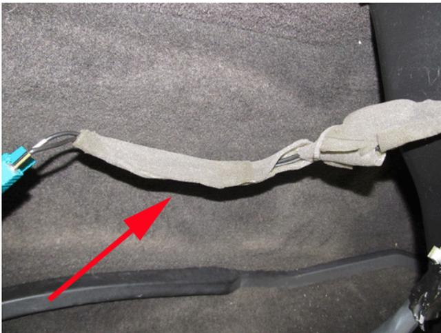
8. Wrap the female to male cable and the UHF adaptor cable with 3M™ 4314 Urethane Foam Tape or equivalent to eliminate any potential noise as shown above.
