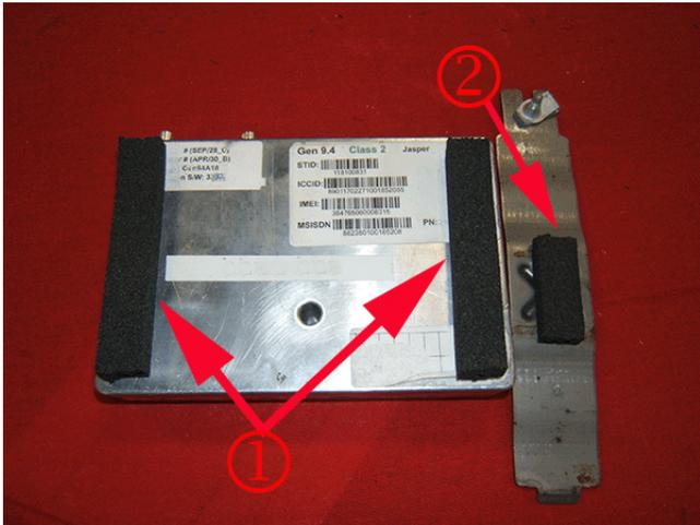
Install two strips of Kent Automotive Adhesive-Back Shim Stock 3/4" Wide X 7/16" thick or equivalent to the bottom of the OnStar® module and install a piece of foam (2) to the locking strap as illustrated.
