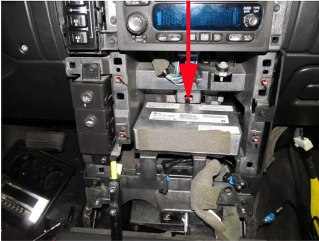
12. Secure the module to the recently installed Velcro® 191195 Reclosable Loop Fastener Tape (hook and loop) or equivalent inside the I/P as shown above. Ensure to position the cables out of the way of the module while installing.
