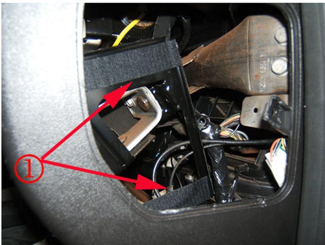
Install the other side of the 2" Velcro® 191195 Reclosable Loop Fastener Tape (hook and loop) or equivalent to the OnStar® module bracket as illustrated.
