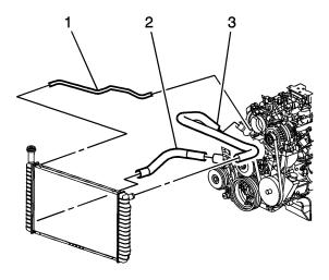
Remove the radiator vent inlet hose (1) from the radiator.
