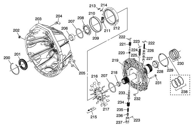
Disassemble the pump to inspect the turbine shaft front bushing (218). If the bushing is damaged, replace the pump cover and the 4-5-6 (w/Turbine Shaft) Housing Assembly (441).
