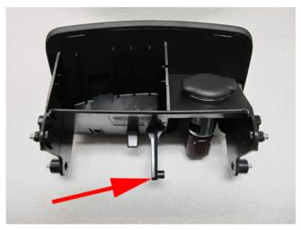
4. Inspect the arm on the back of the compartment for damage.
