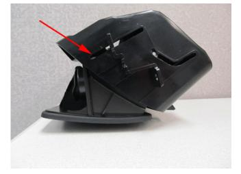
This may be caused by the front floor console rear compartment alignment pins becoming unseated. This can occur if the rear compartment is pushed or kicked.
