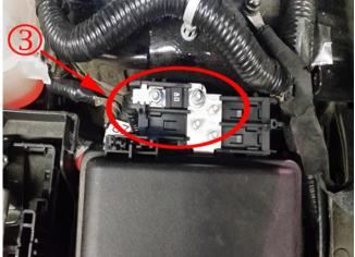
1. Inspect the G111 ground (1) and the 100A F3UB fuse (2) (LaCrosse, Regal, Impala) or 80A F72UA fuse (3) (XTS) for proper connection. Ensure the ground is free of paint and both connections are tight.
