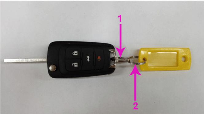
**Notice:** ONLY the key with integrated fob should be on the first 19 mm (16 mm ID) ring (1).
