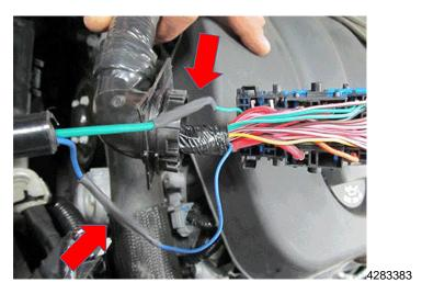
19. Splice the new fan relay control wires from new harness (D-GN and D-BU) to the matching cut wire ends leading to PCM. Apply heat to the heat shrink tubes to seal the splices.
