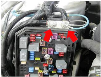
14. Remove the nuts from both UBEC battery studs, and remove all ring terminals. The convoluted conduit on the left ring terminal may not be present in some vehicles. It may appear as double-crimped fusible links to a single ring terminal.
