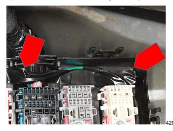
21. Use electrical tape to keep the two wire leads in place during UBEC re-installation.
