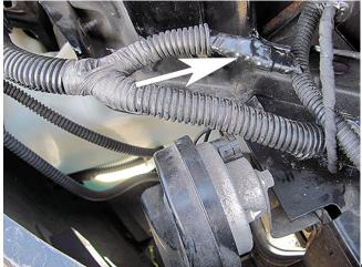
6. Seal the four cut leads of the harness with four Duraseal Splice Tubes. Wrap the cut harness section with electrical tape to prevent moisture damage.
