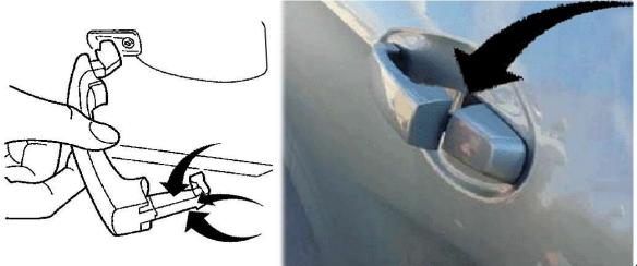
Lubrication points (arrows) on door handle unpainted black tower leg. (Exploded view shown for detail, disassembly not required.)
