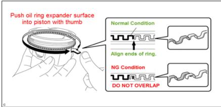
Using a piston ring expander, install the No. 1 compression ring and No. 2 compression ring with the code mark positioned as shown in the illustration.
