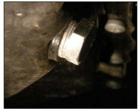
If the oil pan has a boss use part number: N 908 132 02 Drain plug w/seal
