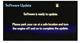
E. Do not remove the USB Drive SST or turn Off the ignition until the navigation screen is present.
