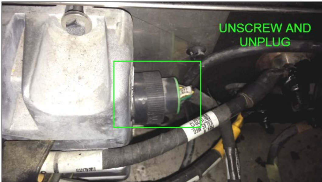
Fig.8 Equalizer side connection & harness
