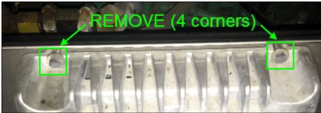
Fig.9 Equalizer top mounting hex bolts
