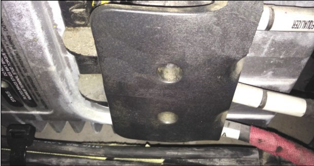
Fig.13 Reinstalled wire cover
