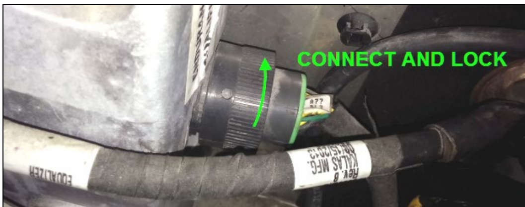
Fig.10 Reconnecting Equalizer harness
