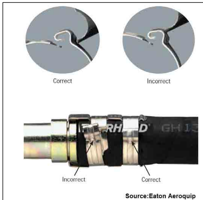
Figure 13 : Clamp ring clasp recommendations
