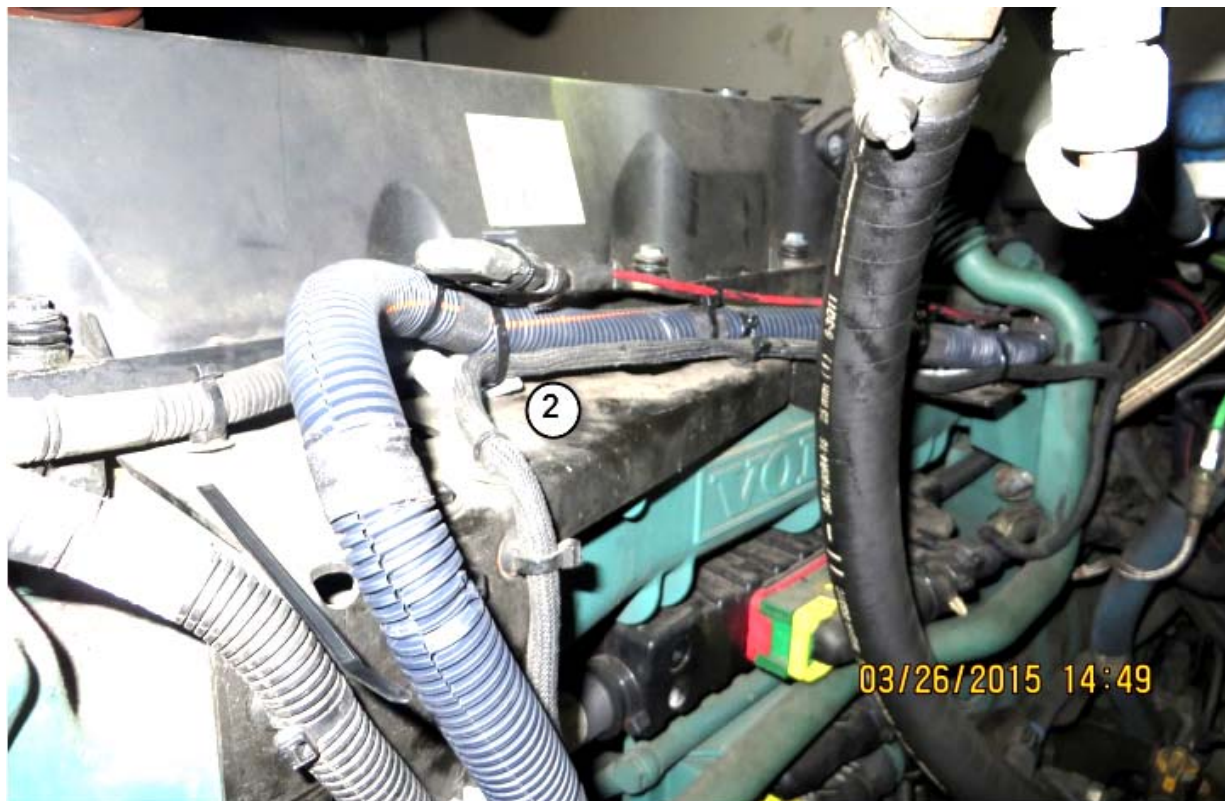
FIGURE 14: POWER CABLE ATTACHED TO #2 DOUBLE-TIE MOUNT AND PROPER NYLON TIES INSTALLATION
