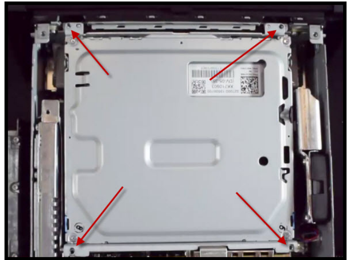
Figure 11. CD drive mounting points are now free.
