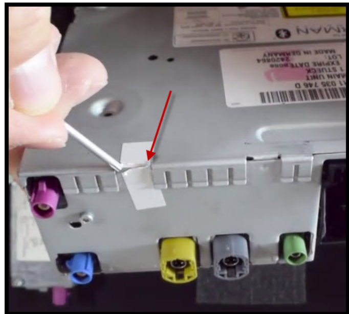
Figure 7. Break the white warranty seal.
