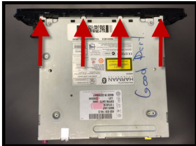
Figure 9. Top cover metal tabs indicated by the red arrows.
