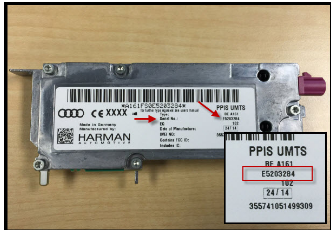
Figure 14. Serial number of the PPIS UMTS telephone module indicated by the red arrows and red box.
