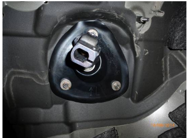
Figure 2. C7 sealing sleeve on the bulkhead.
