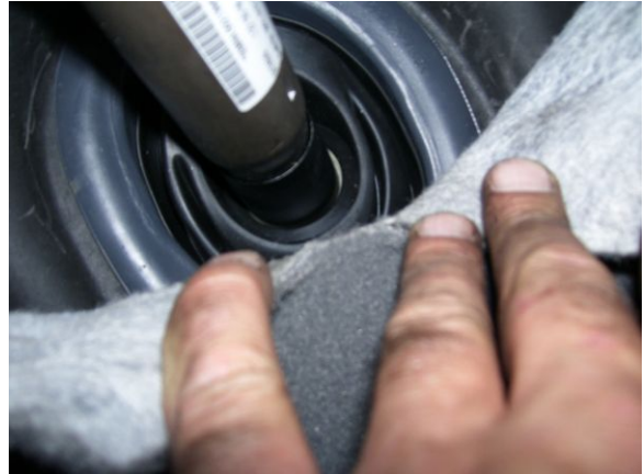
Figure 1. B8 sealing sleeve on the bulkhead.
