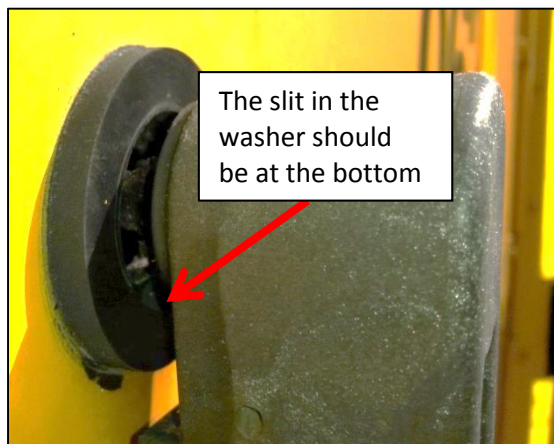
Figure 5, Position of Slit in Washer
