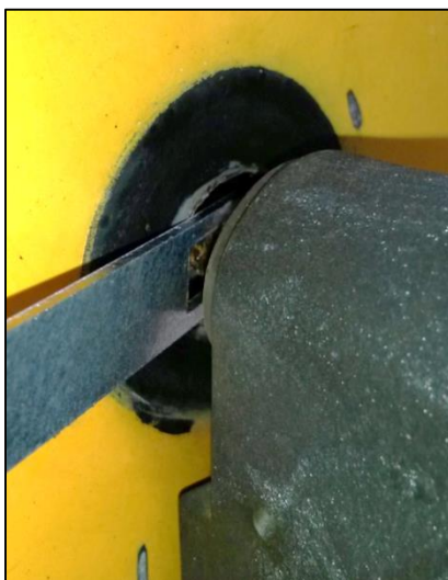
Figure 3, Using the Go/No Go Gauge
