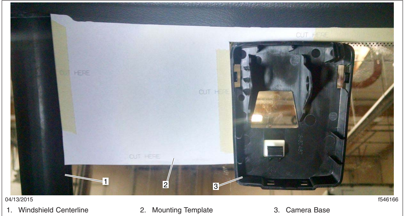
Fig. 6, Mounting the Camera Base using the Template
