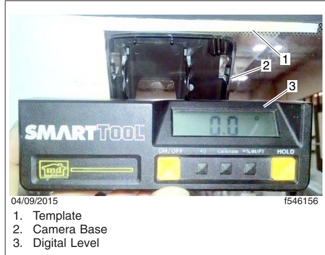
Fig. 8, Aligning the Base with a Digital Level
