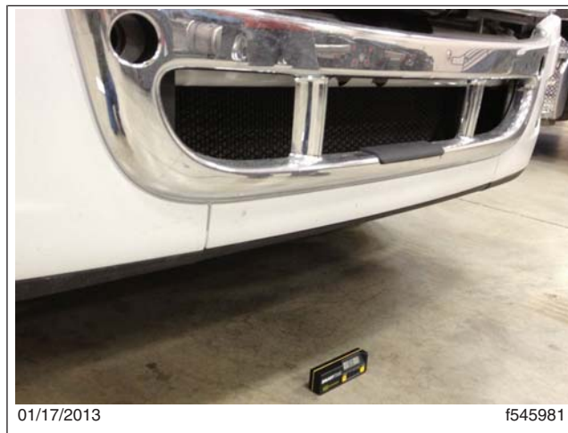
Fig. 5, Measuring the Level on the Surface where the Vehicle is Parked
