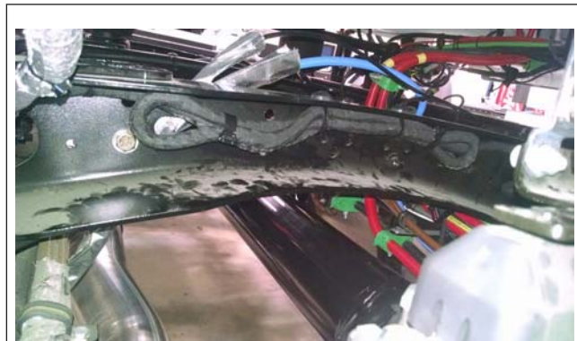
Fig. 6, Harness Secured in the Crossmember with nylon Cable Ties, Part Number 23-12069-001
