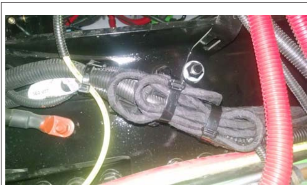
Fig. 5, Excess Harness Secured
