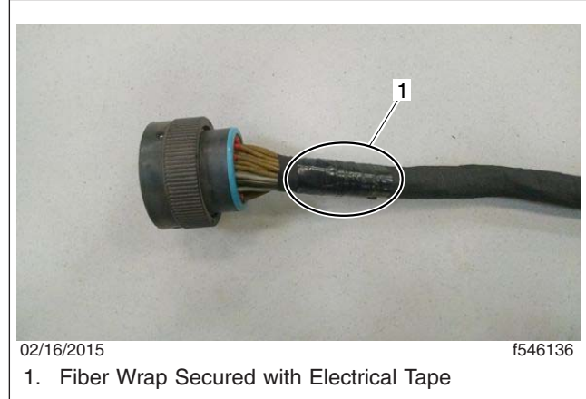
Fig. 15, Fiber Wrap Secured with Electrical Tape
