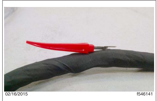
Fig. 10, Cutting the Fiber Using the Blunt End of the Seam Cutter
