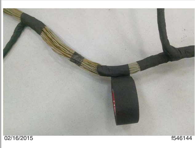
Fig. 14, Wrapping the Harness with Fiber Tape
