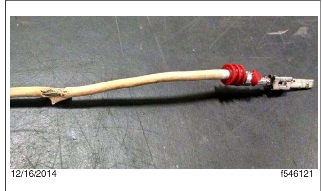
Fig. 2, Insulation Discoloration, Major
