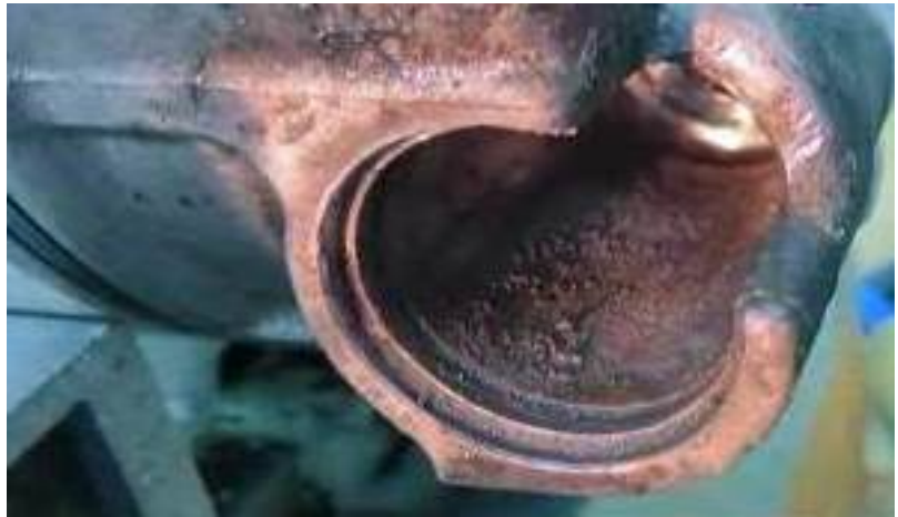
Figure 10. Corrosion in the N280 valve bore.
