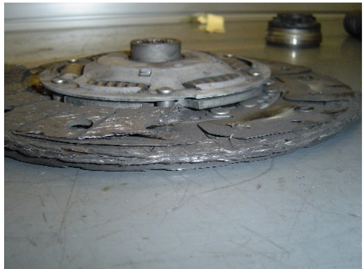
Figure 2. Burst lining from an overspeed condition.
