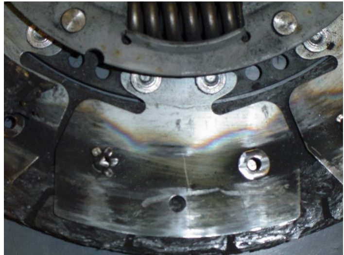
Figure 1. Lining partly removed due to overheating.
