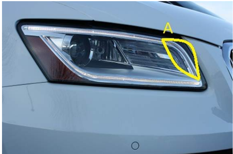
Figure 5. Upper light pipe perceived defect (A).
