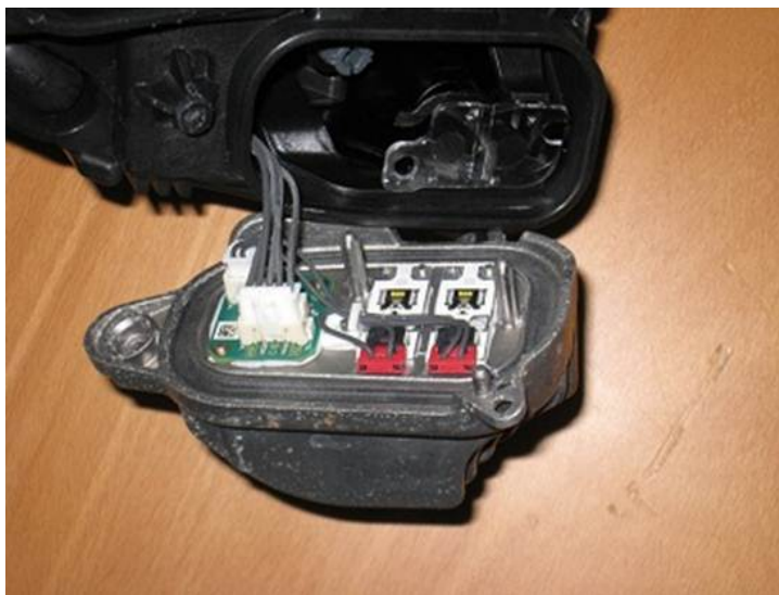
Figure 7: Dual surface mount LED unit exposed.
