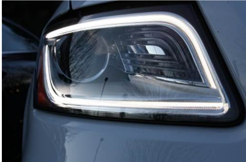
Figure 1. Upper and Lower light pipes illuminated.
