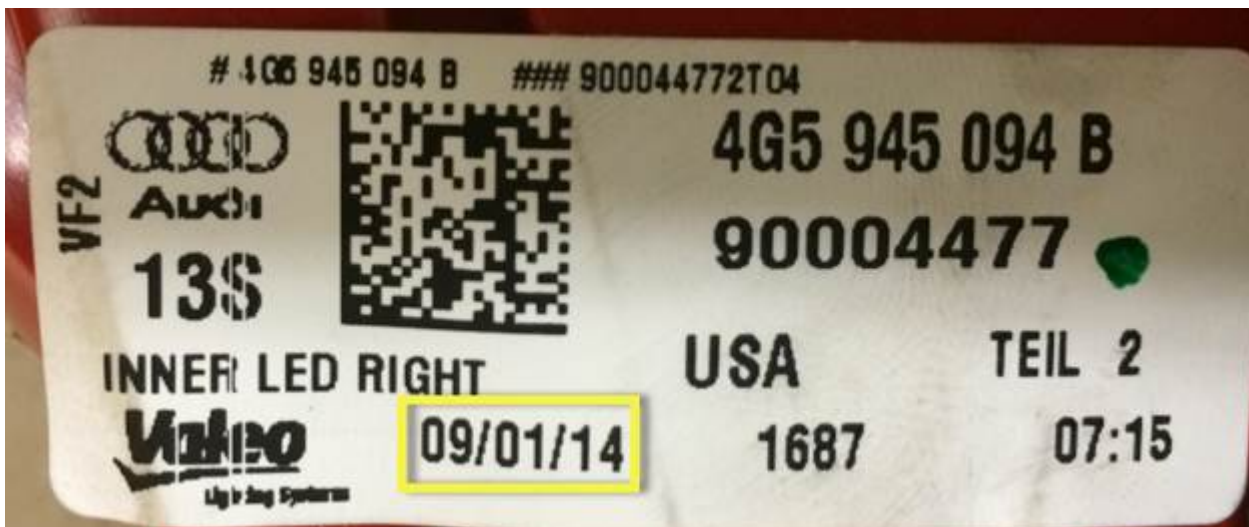
Figure 2. Location of production date, shown as DD/MM/YYYY. The production date of this taillight is January 9, 2014.
