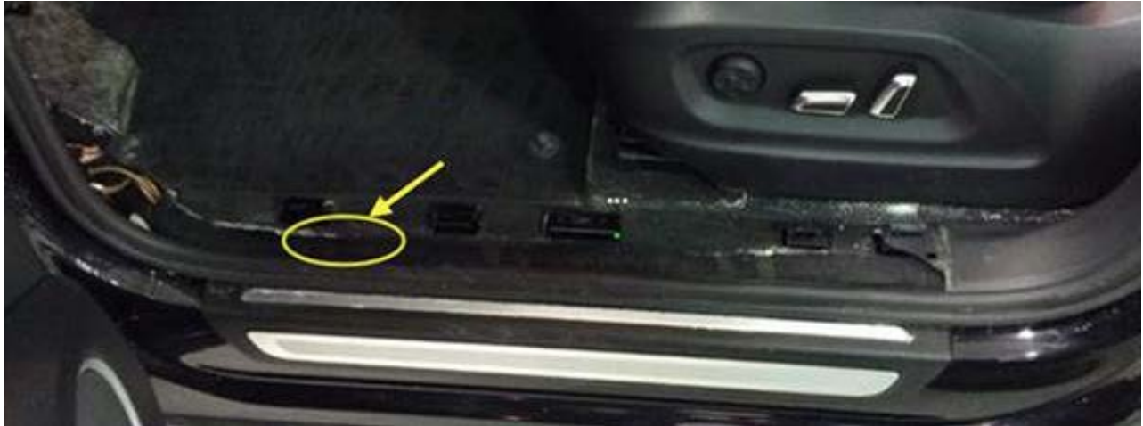
Figure 8. Open the wiring harness.
