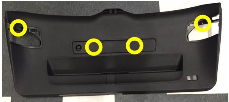
Figure 1. Screw location on lower tailgate trim.
