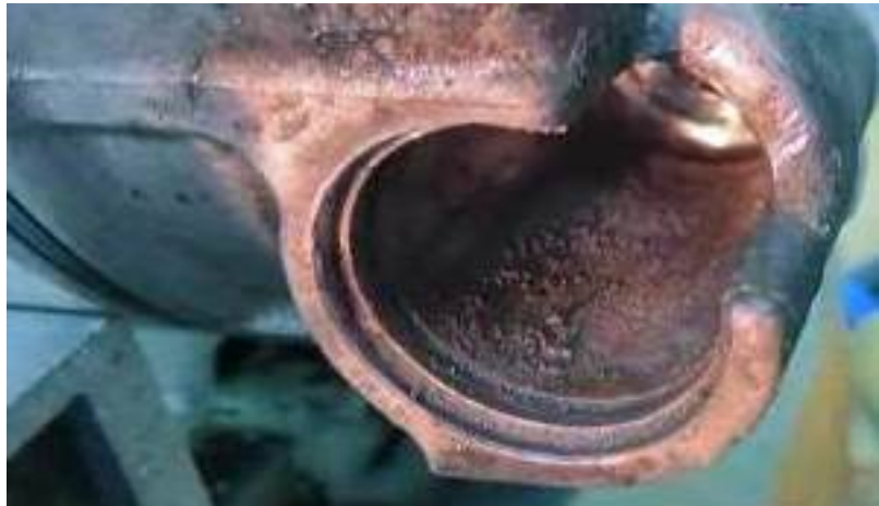
Figure 10. Corrosion in the N280 valve bore.
