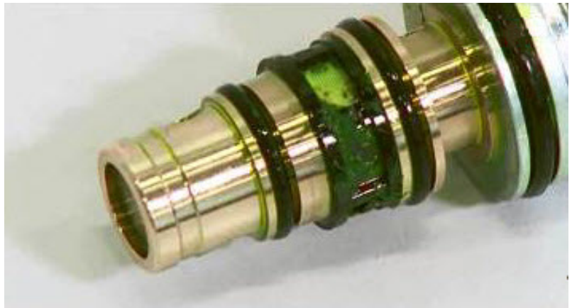
Figure 11: Severe contamination at the N280 valve filter screen.
