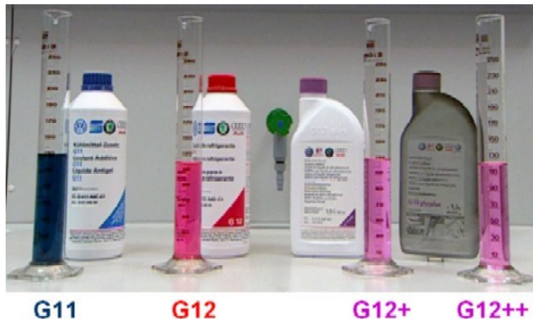
Figure 1. The color of each type of engine coolant. G11 (green-blue), G12 (red), G12+, G12++ and G13 (purple).
