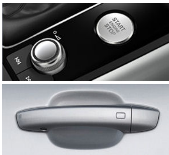
Figure 1. Start-stop button and door handle with touch sensor surface.
