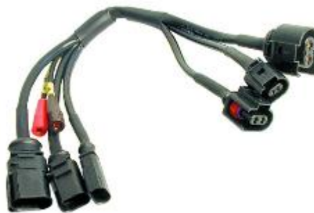
Figure 7. VAS 5256 breakout harness.
