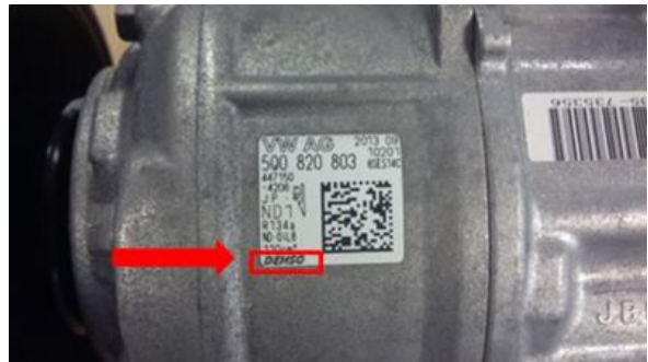
Figure 14: Denso compressor identification tag.
