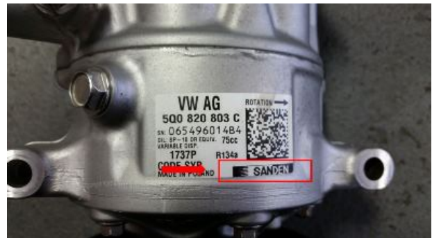
Figure 3. Sanden compressor identification tag.
