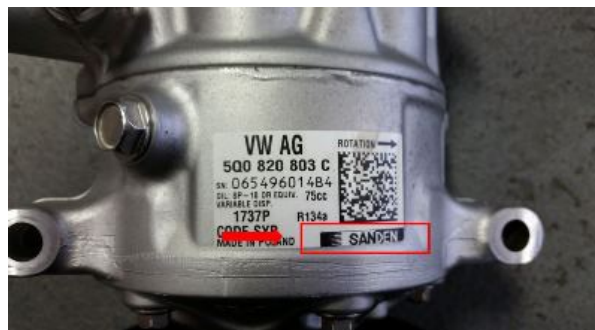
Figure 13: Sanden compressor identification tag.
