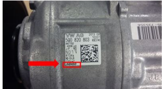
Figure 2. Denso compressor identification tag.
