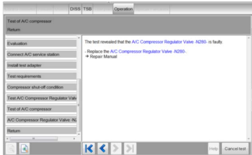
Figure 12: Test plan confirming that the N280 is faulty.
