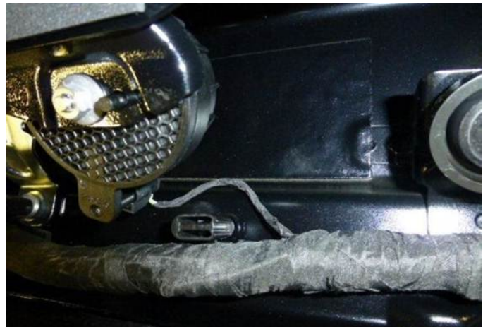
Figure 3. Sound actuator R214 in the plenum chamber.
