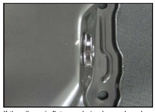
If the oil pan is flat, use drain plug and washer:
