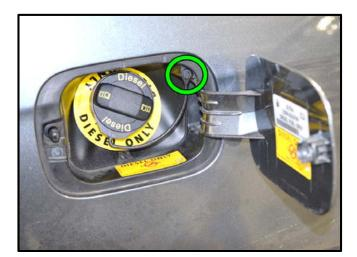
C The retaining ring is installed into the filler neck with the alignment pins <circles> facing toward the fuel tank.
