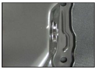
If the oil pan is flat, use drain plug and washer: N 911 679 01 Plug N 013 81 57 Seal
