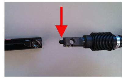
3. If not present in the upper I-Shaft, check down the inside of the lower I-Shaft and joint for the plug. Invert the shaft and while manipulating the joint strike the open end downward on a shop towel on a workbench. If found, remove the plug, discard and reinstall the lower shaft.
