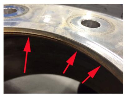
This is caused when the wheel is not centered on the hub and is then forced over the hub extension centering lip during torqueing of the wheel. These wheels MUST be manually tightened down to properly center the wheel on the hub before torqueing. If this condition is found, replace the affected wheel.
