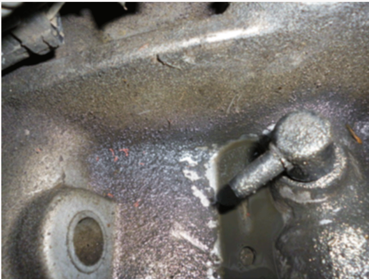
Figure 2. Breather Vent Location
