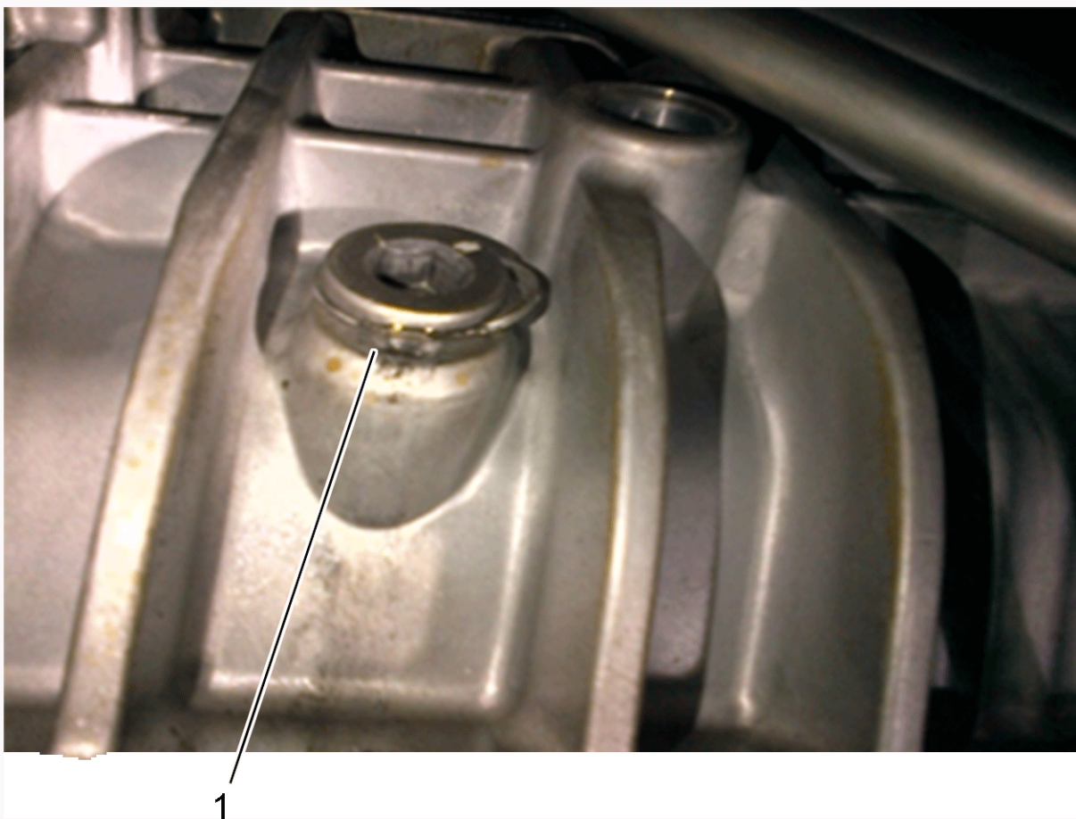
Figure 10. Cross-threaded Oil Fill Plug
