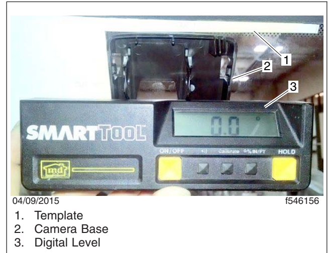
Fig. 9, Aligning the Base with a Digital Level
