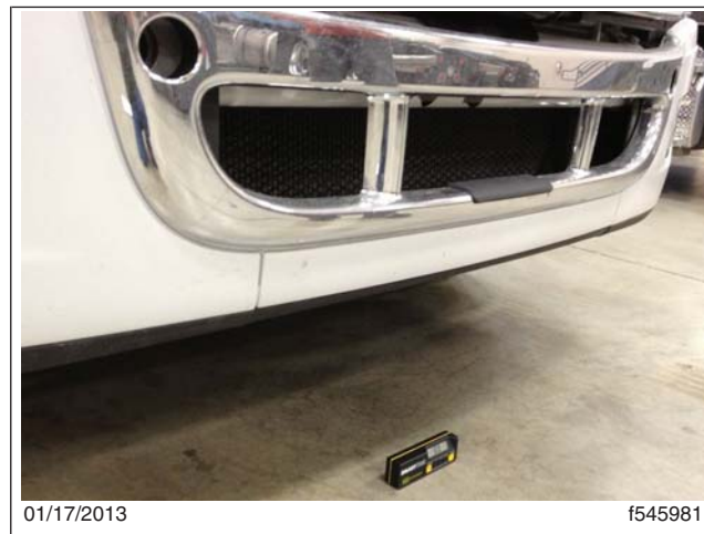
Fig. 6, Measuring the Level on the Surface where the Vehicle is Parked
