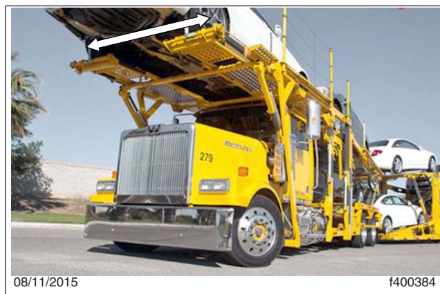
Fig. 1, Centering the Vehicle Over the Cab
