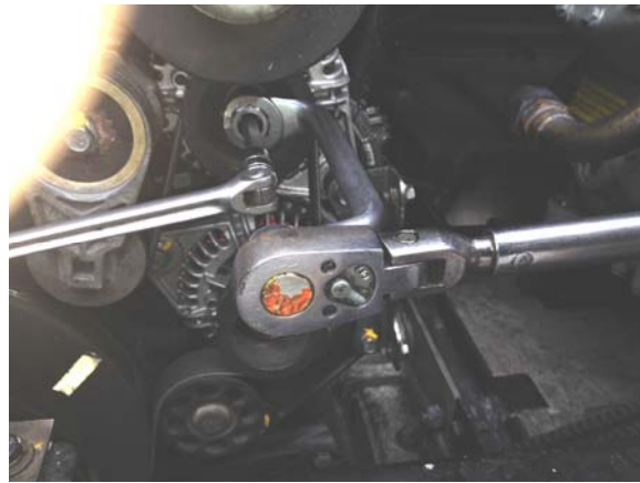
OFFSET 7/8 WRENCH FITTED WITH 7/8 SOCKET AND 10mm 12-POINTS SPLINE DRIVE
