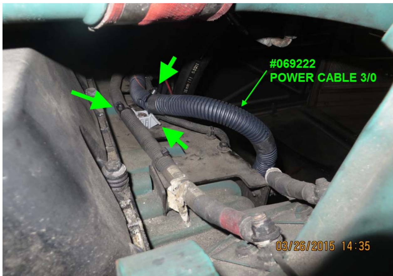
FIGURE 11: POWER CABLE ATTACHED TO #2 DOUBLE-TIE MOUNT AND PROPER NYLON TIES INSTALLATION
