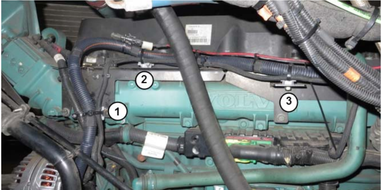
FIGURE 9: POWER CABLE ATTACHED TO #1, #2, #3 DOUBLE-TIE MOUNT AND PROPER NYLON TIES INSTALLATION
