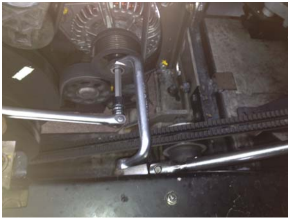
USING THE CYLINDER HEAD WRENCH WITH A RATCHET DRIVE AND A FLEX SOCKET WRENCH
