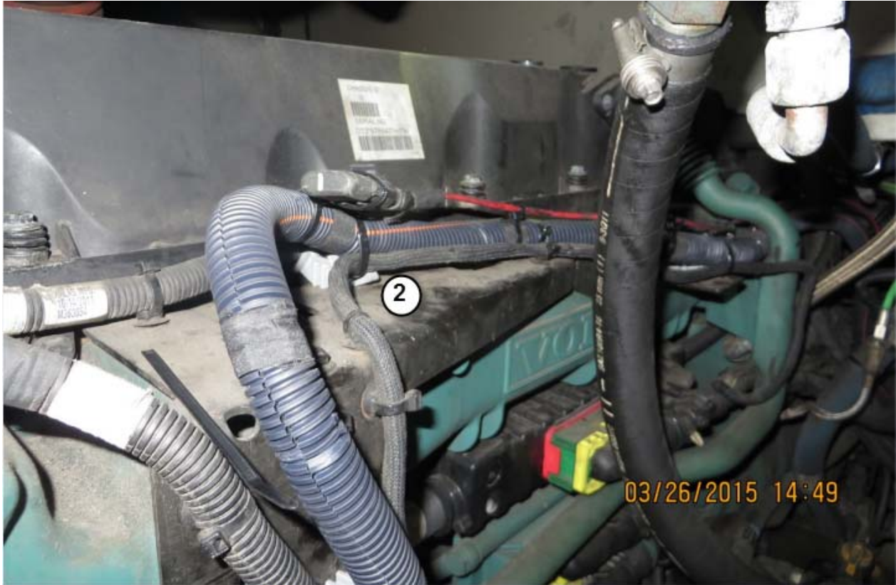
FIGURE 12: POWER CABLE ATTACHED TO #2 DOUBLE-TIE MOUNT AND PROPER NYLON TIES INSTALLATION
