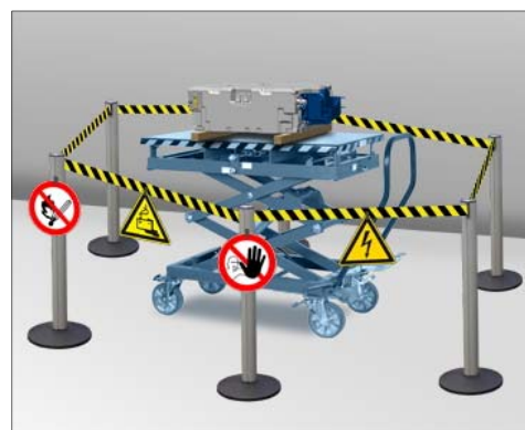
Restricted area for HV battery
