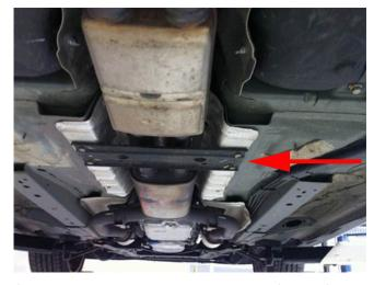
GM does not support permanent removal or modification of the brace as it would result in degradation of the side impact and N&V performances of the vehicle.
