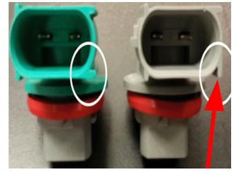
If you encounter a vehicle with the above concern, use a piece of sand paper or equivalent to sand the guide pin off to correctly fit the body harness.
