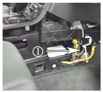
**5.** Locate the large X340 connector (1) with the white lever action CPA. Uncouple the connector.
