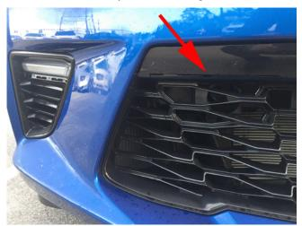
**Note:** Some models you need to carefully open the cover in the front grille by using the small notches located along the top of the grille that conceals the tow eye socket. Use care to not damage the paint or the grille.
