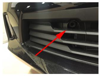
**3.2.** Locate the tow eye socket on the right side of the vehicle in the lower front grille.
