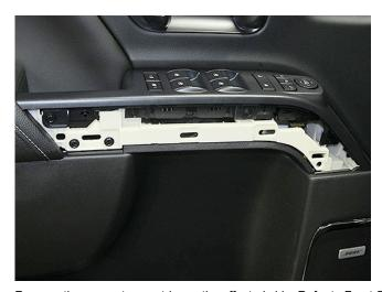
1. Remove the armrest cover trim on the affected side. Refer to Front Side Door Armrest Cover Trim Replacement (With A31) in SI.
