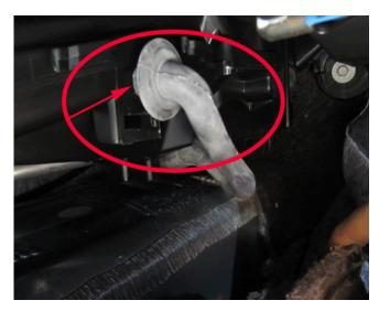
**Note:** Shown in the illustration above is where the plant temporary installs the A/C hose during Instrument panel installment. Do not drill out the temporary holder for any reason.
