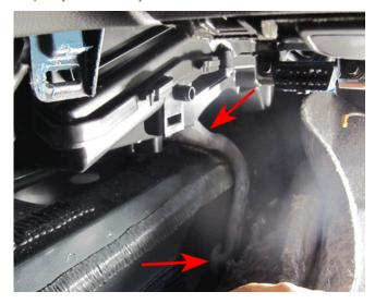
Note: Shown in the illustration above is the A/C hose properly installed onto the correct drain port.
