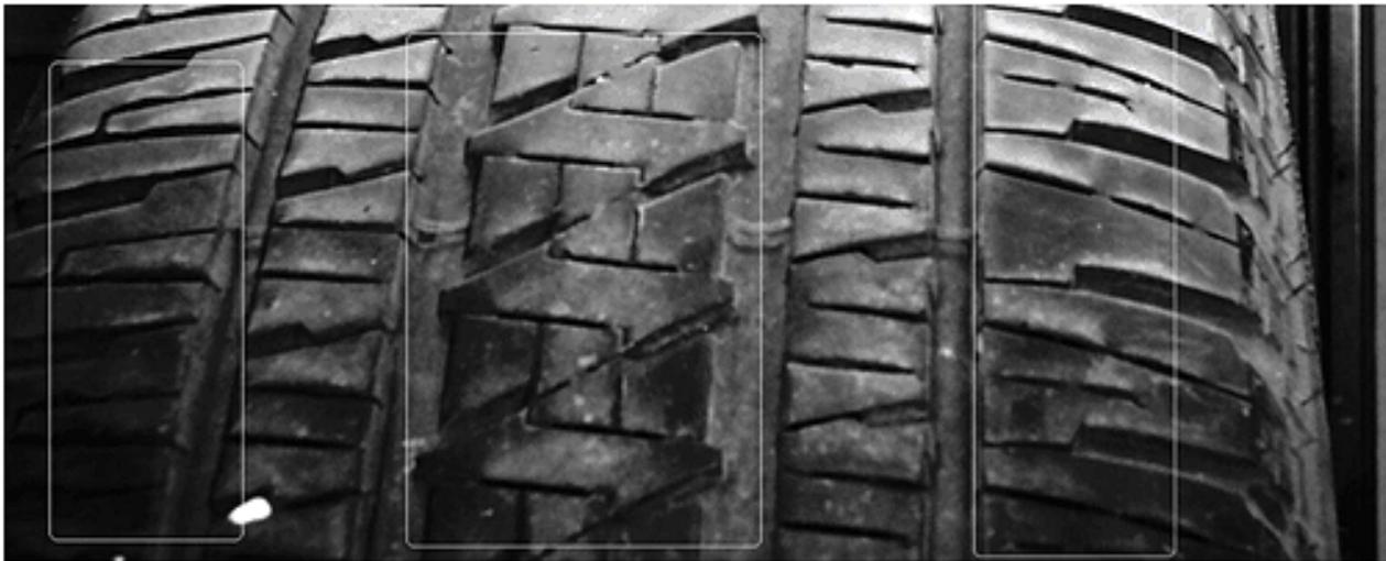
**Figure 2: Tire Shoulder View Example 1 - “NORMAL” Tire “Feathering” Wear on the Shoulder**
