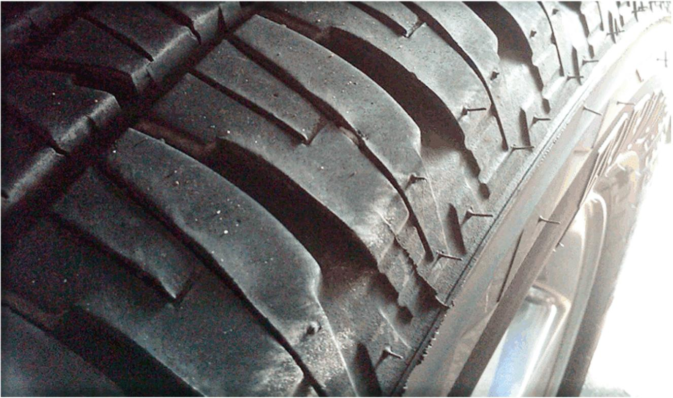
Figure 3: Tire Shoulder View Example 2 - "NORMAL" Tire "Feathering" Wear
