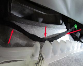
**4.** Reroute the RCDLR harness away from the opening for the rear HVAC duct on the headliner.
