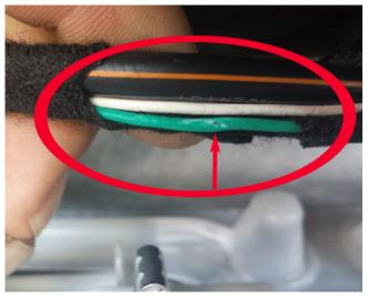
This condition may be caused when the low speed LAN wire to the remote control door lock receiver (RCDLR) becomes pinched between the plastic rear HVAC headliner duct and the roof.
