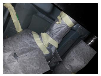
5. Wrap and tape off transmission, transfer case, propeller shaft, cables, wiring, exhaust, etc.to protect from overspray as illustrated above.
