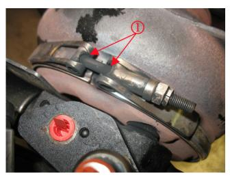
If DTC P003A is found as Current or in History, OR there is evidence of soot leakage (1) in the area of the V-band clamp (1), then technicians MUST verify if the engine control module (ECM) has a Power-Up Kit aftermarket calibration installed or an aftermarket hardware device has been installed.
