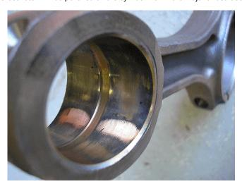
• Piston pin bore will show signs of scoring, the wrist pins will be discolored, and can have oil coking on them. The connecting rod bushing surface will have accelerated wear. The above illustration shows a connecting rod bushing.
