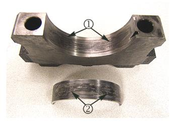
• Signs of bearing fretting will also be noticed on the connecting rod and main bearing caps. Refer to the above illustration for fretting of main bearing cap 1 and back side of connection rod bearing 2.
