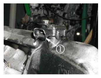
• Excessive heat in engine compartment caused by overpower device. Refer to above illustration (1).
