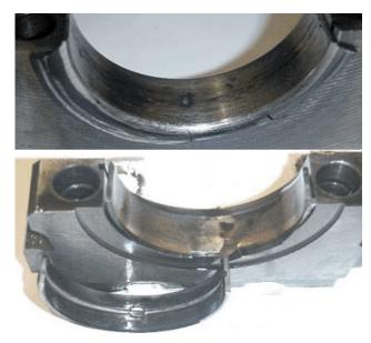
Bearing failure. Spun main bearings.
