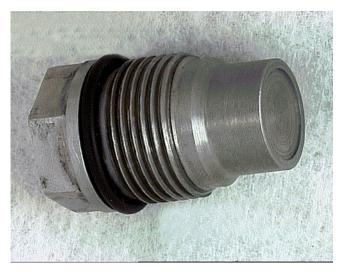
Aftermarket companies have developed a performance pressure relief fuel valve for Duramax<sup>™</sup> diesel engines. Refer to above graphic illustration. The performance pressure relief fuel valve attaches to the fuel rail in place of the OEM valve and will not allow any fuel return to the tank, giving 100% of the fuel to be available for additional engine performance. This may cause additional fuel related driveability concerns and may set the following DTCs:
