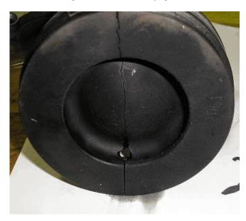
• Pistons will be cracked in the lip area, or a hole in the pistons.
