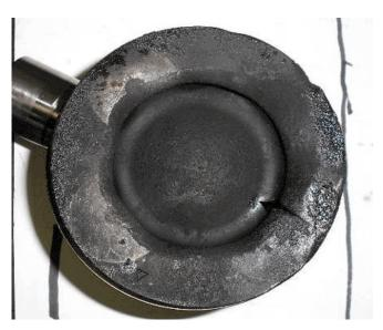
• Pistons can also be melted on the lip of the combustion bowl, or the top of the pistons can be melted.
